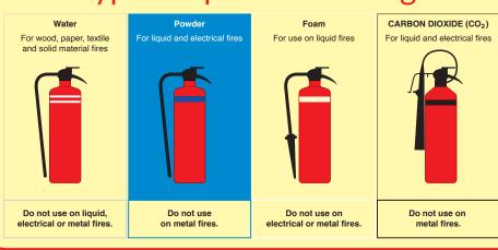
You can see the contents of an extinguisher by looking at the colour on the red body.
